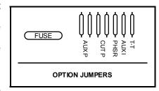
**Auxiliary Input Function** - The auxiliary input normally activates the Horn function. To activate the Man/Phsr function with the auxiliary input cut the jumper resistor labeled "AUX I".
